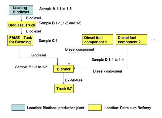
Fig. 1: Diagram of sampling points at Total Deutschland GmbH (supply chain 1)
