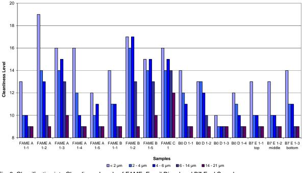
Fig. 3: Classification into Cleanliness Levels of FAME, Fossil Diesel and B7 Fuel Samples
