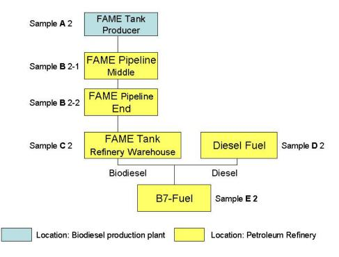
Fig. 2: Diagram of sampling points at OMV Refining & Marketing GmbH (supply chain 2)
