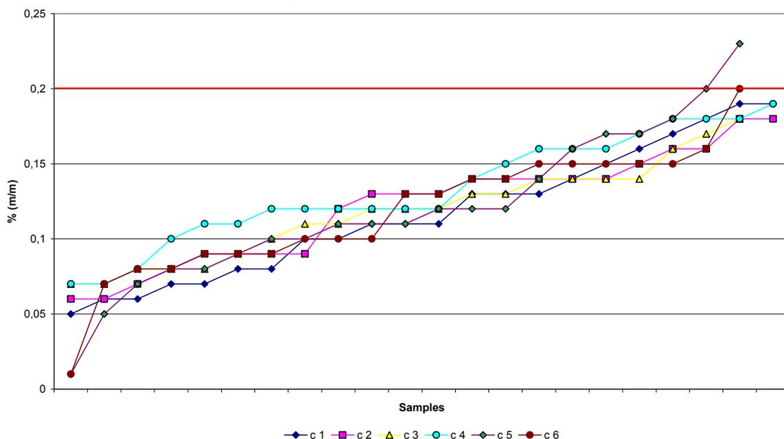
As it is the case with monoglycerides, the graph reflects that the Biodiesel producers have the transesterification process under control. Failure and ensuing exceedance of limits almost only occur when the plants are started and/or in case of technical faults. Generally such problems are detected during in-house operational checks. Despite the fact that the limit was exceeded in one single case, the standard was observed in all cases considering the precision of the test method.
