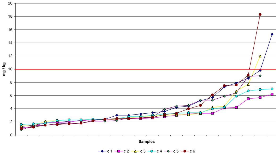
Three samples of the last six campaigns show sulphur values of above the limit. In two cases the cause for that was identified as increased use of sulphuric acid ( $H_2SO_4$ ) during production, in the third case the cause could not be finally resolved. Appropriate corrective measures were taken.
