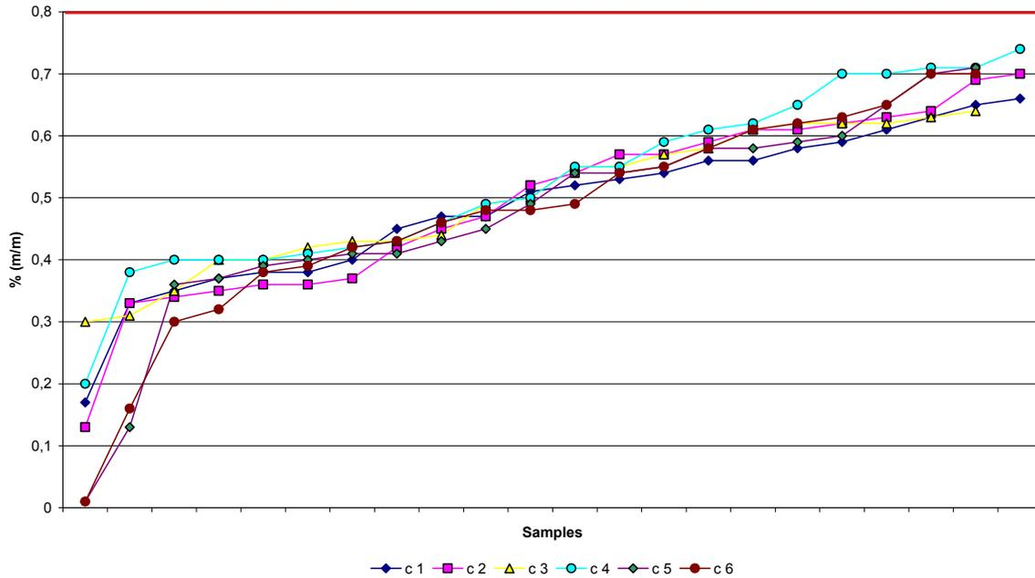
FAME according to DIN EN 14214 may contain a maximum of 0.8 % (m/m) of monoglycerides. The graph shows that all tested samples stay below the limit and that most producers are already in a position to meet the lower limit for FAME as pure fuel of 0.7 % (m/m), which will take effect with the next revision of DIN EN 14214.
