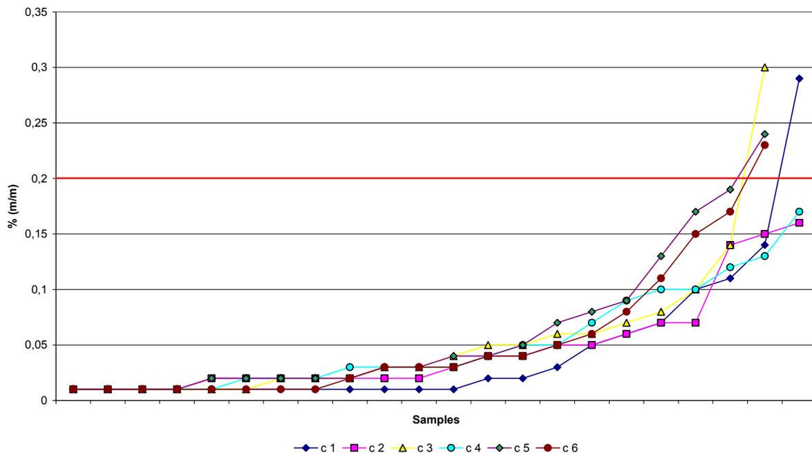
Again the evaluation shows that generally the contents are way below the permissible values and in most cases they are even below the determination limit of test method DIN EN 14103. The commodities of the two detected violations were not delivered and corrective measures were taken; considering the precision of the test method the limit was just observed in two cases. Limits are exceeded, with a simultaneous increase of diglyceride values, primarily in case of production plant failure.
