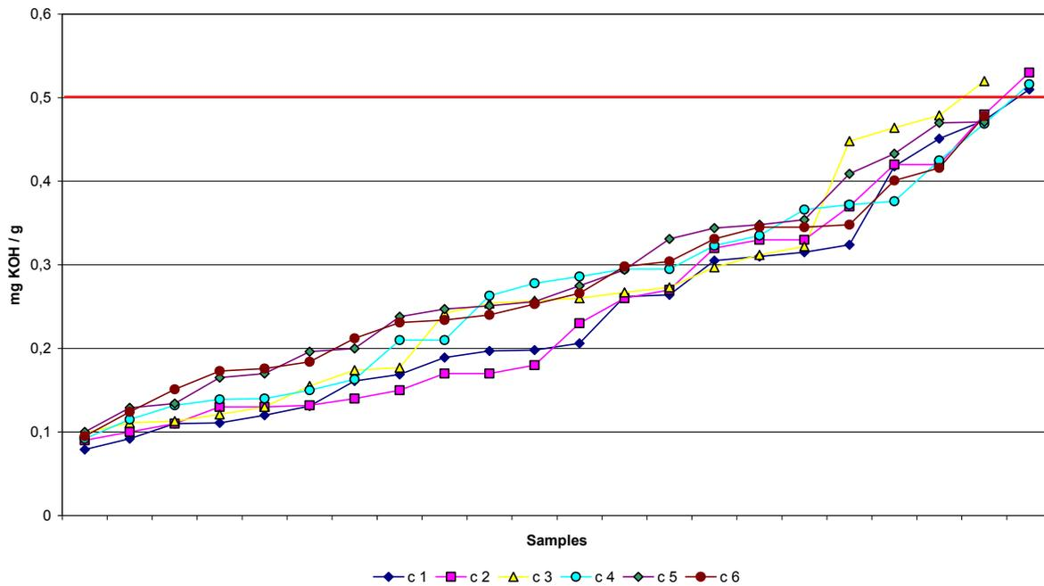
With the exception of four cases the limit of DIN EN 14214 was observed. However, the four exceeding values were so small that with regard to the precision of the test method the standard was observed.
