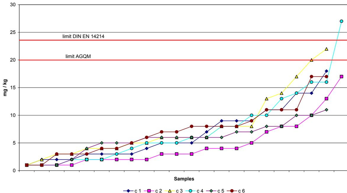
The result of the sampling campaign is pleasing: only two samples exceed AGQM's limit while the majority of samples contains less than 10 mg/kg of 'dirt' by far. Considering the precision of the test method DIN EN 14212 is observed in all cases.
