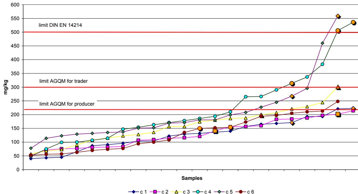
The majority of samples contain less than 200 mg of water/kg which is even significantly below AGQM's stipulation. All results meet the limit of DIN EN 14214 considering the precision of the test method. It is notable that the values of campaigns 4 and 5 are higher than those of the other campaigns and that all those exceeding the AGQM limit of 300 mg water/kg stem from these two campaigns. The reasons for that are the high summery temperatures with increased absolute humidity.
