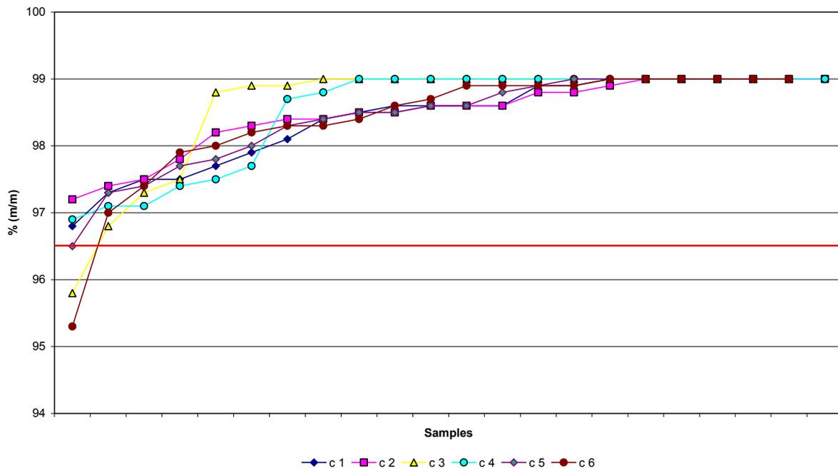
The graph shows that the limit of the standard is observed with the exception of two values. Considering the precision of the test method, all values meet the requirements of DIN EN 14214. Measuring values given as '> 99.0 %' are shown in the graph as ester content of 99 %.
