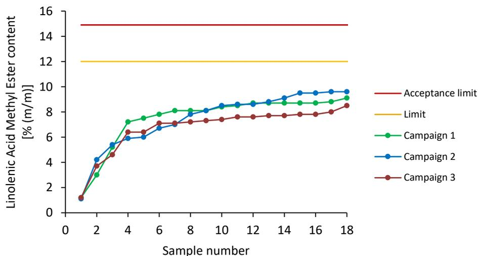
Figure 18: Content of Linolenic Acid Methyl Ester acc. to DIN EN 14103.
