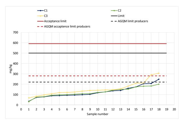
Diagram 4: Water Content acc. to DIN EN ISO 12937.
