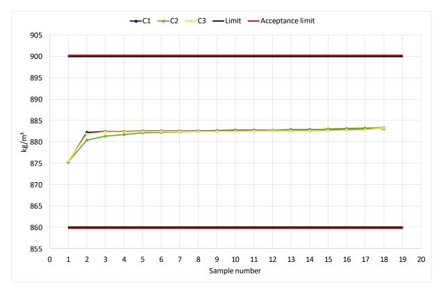
Diagram 2: Density at 15 °C acc. to DIN EN ISO 12185.
