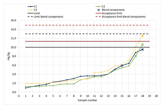
Diagram 3: Sulphur Content acc. to DIN EN ISO 20846.
