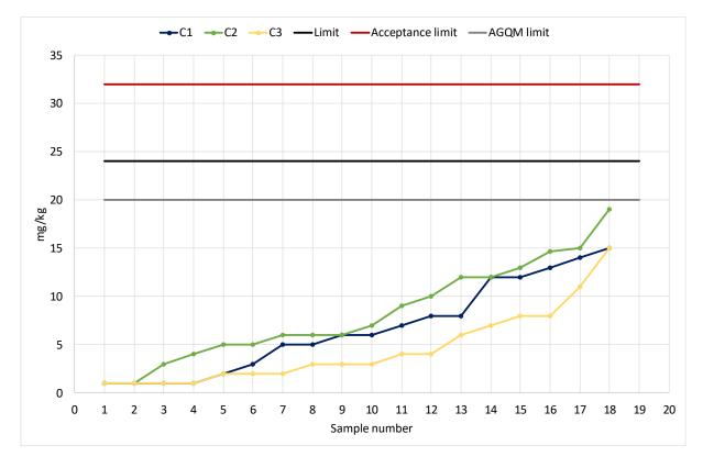
Diagram 5: Total Contamination acc. to DIN EN 12662.
