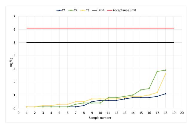
Diagram 13: Sum of Alkali Metals Sodium and Potassium acc. to DIN EN 14538.
