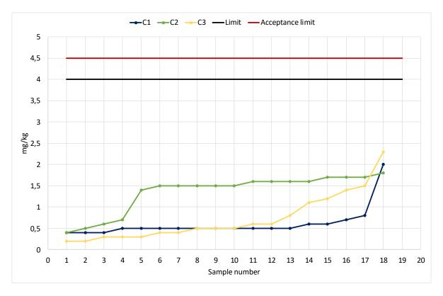
Diagram 15: Phosphorous Content acc. to DIN EN 14107.
