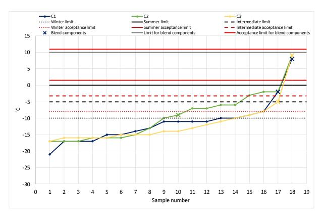
Diagram 17: CFPP acc. to DIN EN 116.
