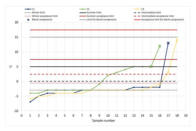
Diagram 18: Cloud point acc. to DIN EN 23015.
