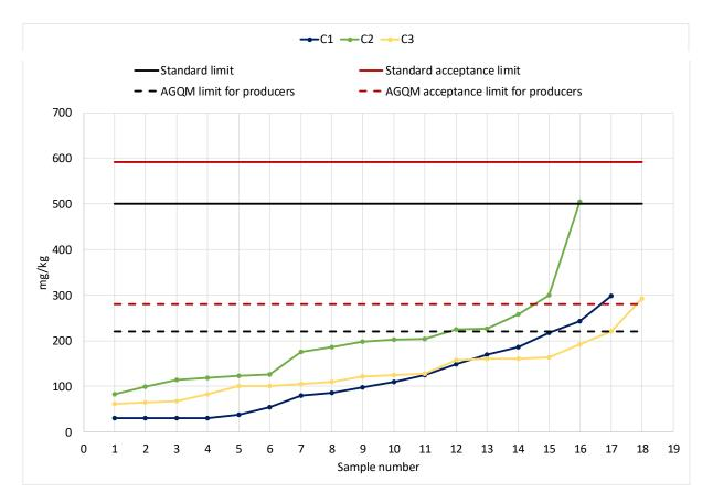
Diagram 4: Water Content acc. to DIN EN ISO 12937.
