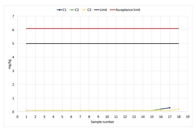
Diagram 14: Sum of Alkaline Earth Metals Calcium and Magnesium acc. to DIN EN 14538.
