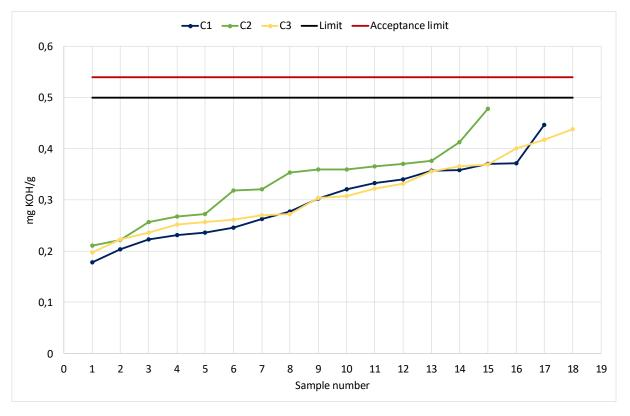
Diagram 7: Acid Number acc. to DIN EN 14104.
