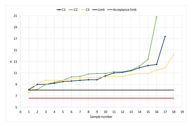
Diagram 6: Oxidation Stability acc. to DIN EN 14112.
