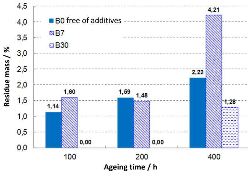
Figure 2-2: Residue mass in aged fuels in dependence on FAME content [3]
