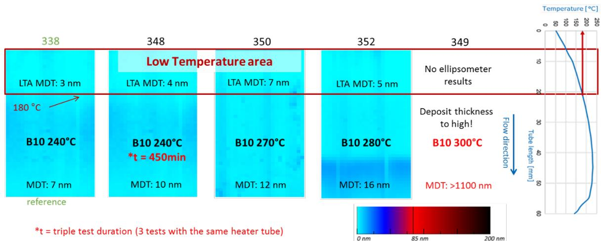
Figure 4-2: Thickness maps and DDFT results for a B10 fuel with extended test period and/or increased test temperatures
