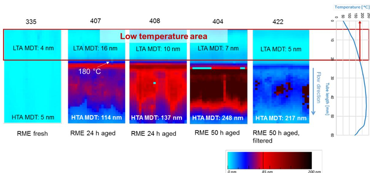
Figure 4-9: Thickness maps and DDFT results – RME ageing on the test bench
