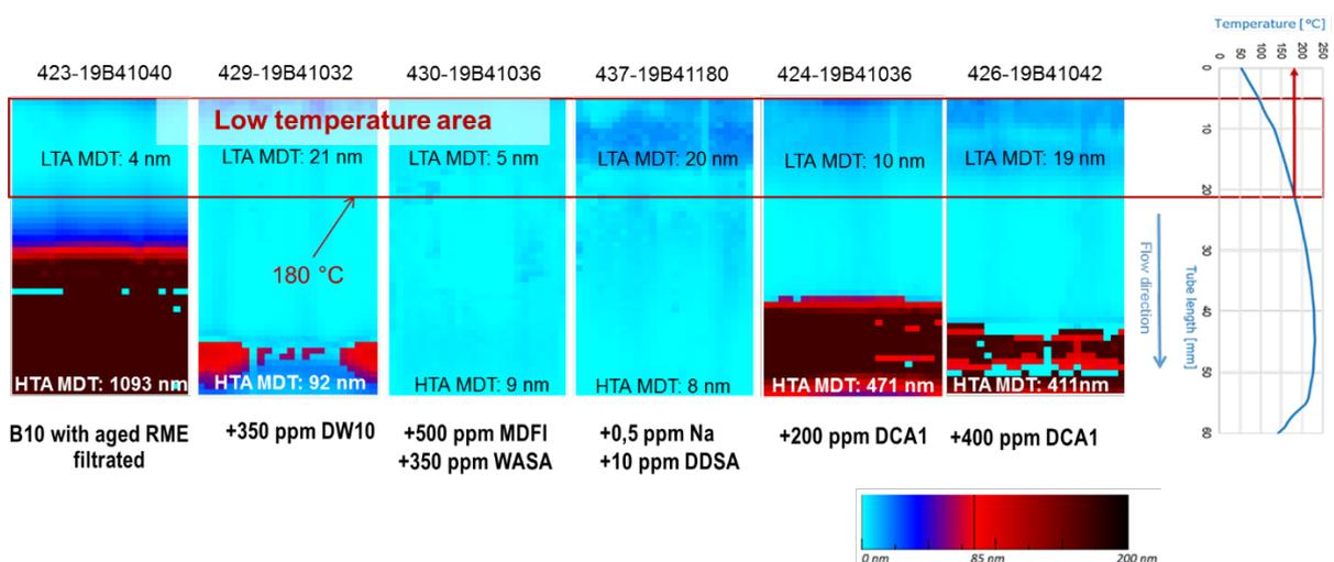
Figure 4-12: Thickness maps and DDFT results – Impact of various additives and saponification agents on the deposit formation of B10
