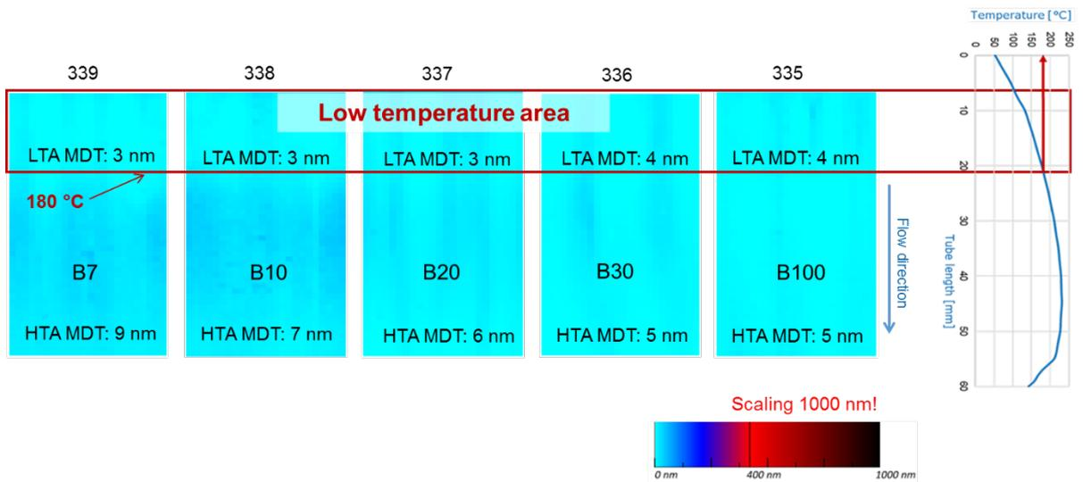
Figure 4-5: DDFT results for various diesel-RME blends at 240°C
