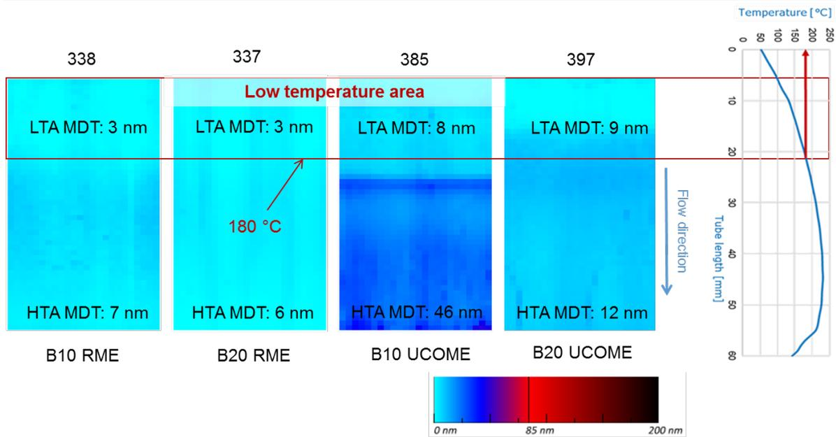
Figure 4-6: DDFT results for various diesel-UCOME blends at 240°C
