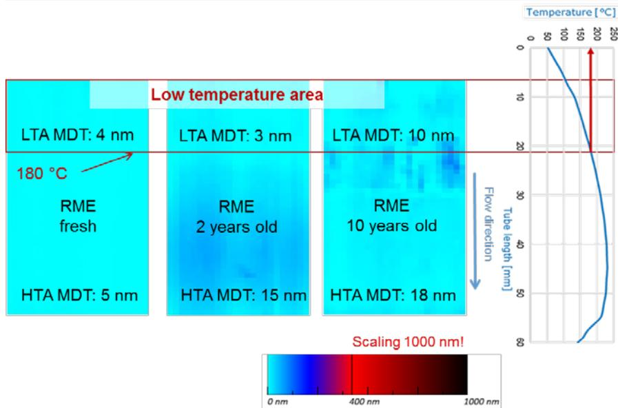
Figure 4-7: DDFT results of naturally aged RME with various storage periods
