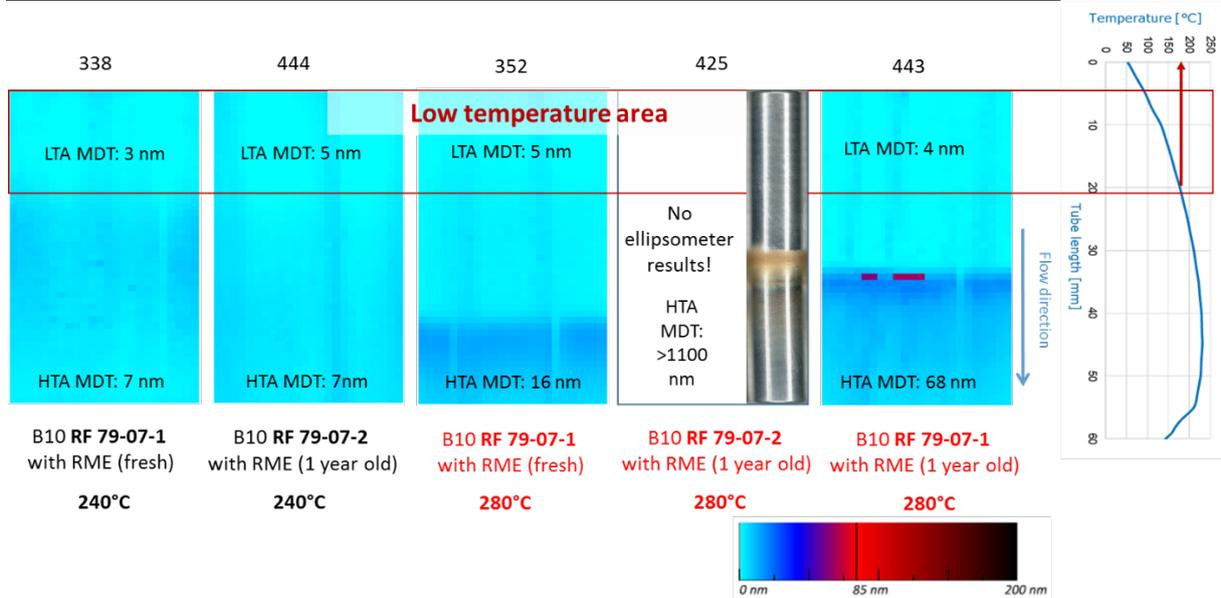
Figure 4-13: Thickness maps and DDFt results – Impact of diesel fuel admixture component and temperature
