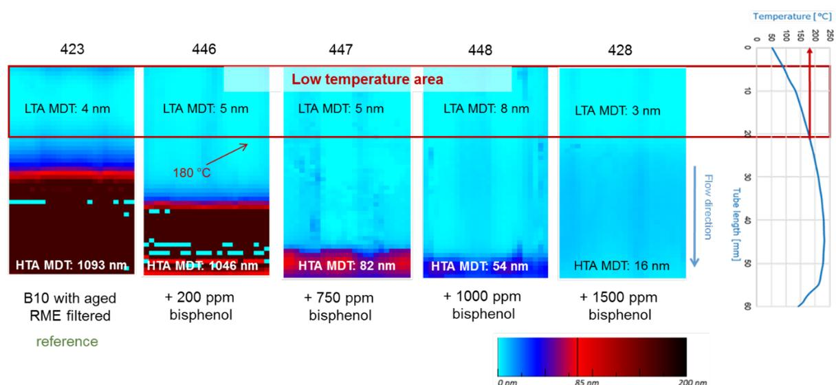
Figure 4-11: Thickness maps and DDFT results – Impact of various concentrations of AO on the deposit formation of B10
