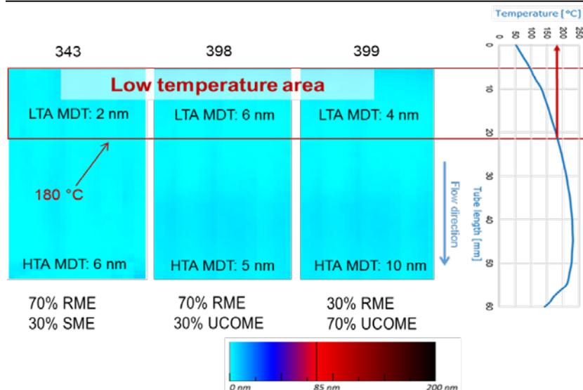
Figure 4-4: : DDFT results for various types of biodiesel at 240°C
