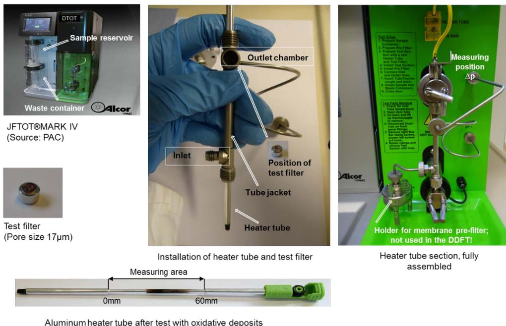
Figure 3-1: Description of the measuring system
