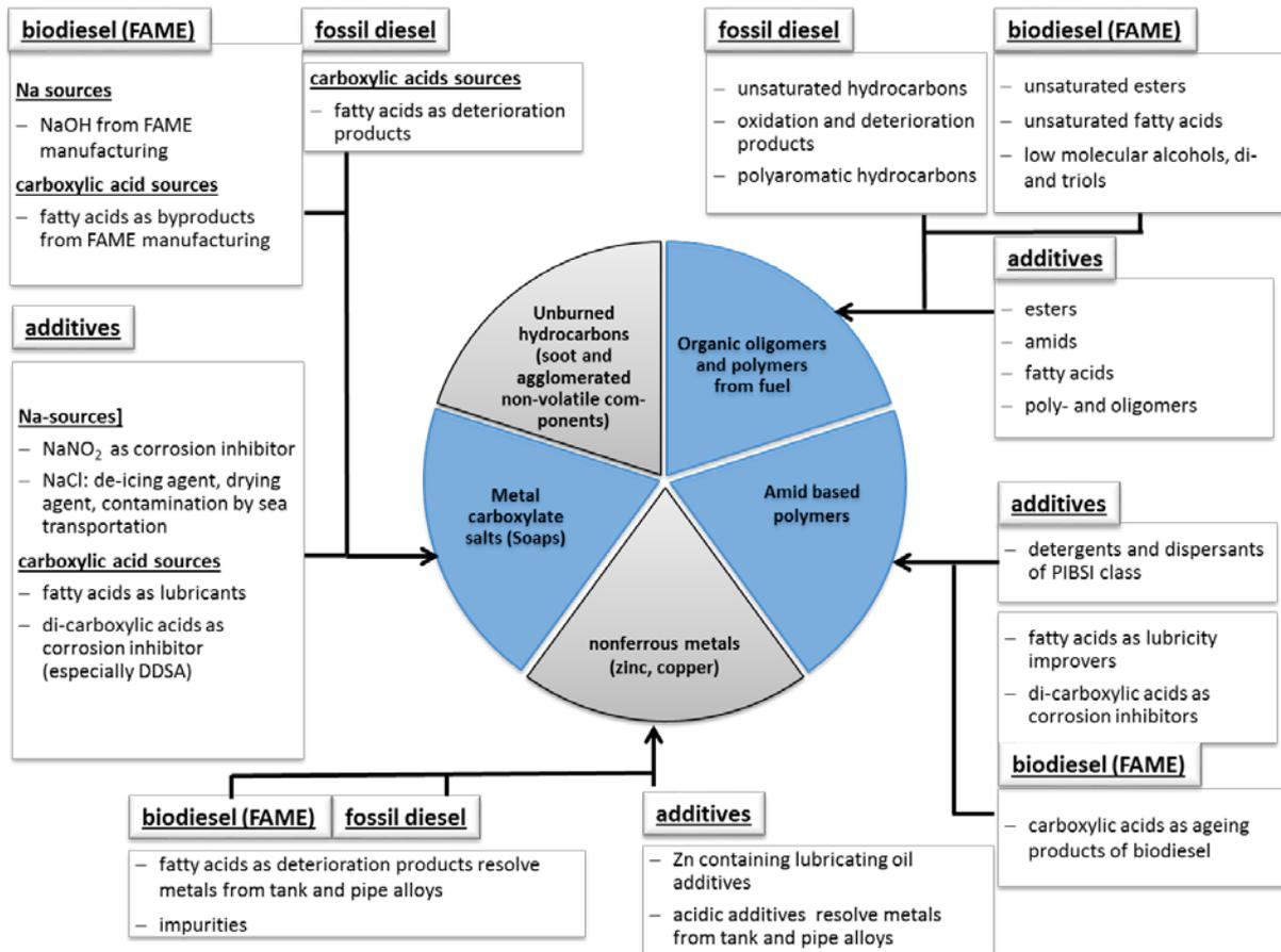
Figure 2-1: Deposit types and sources [3]
