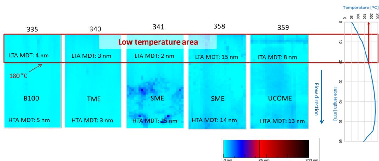
Figure 4-3: Thickness maps and DDFT results of various types of biodiesel
