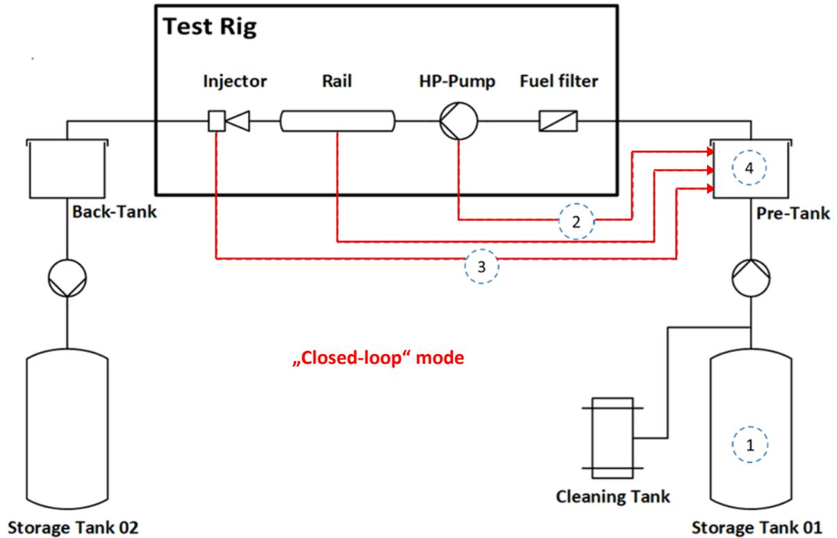
Figure 4-8: Test bench schematic design of an injection system test bench – closed-loop operations
