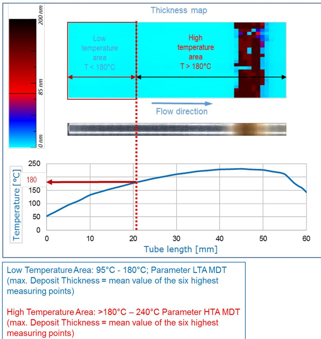
Figure 3-2: Temperature-dependent evaluation of deposits
